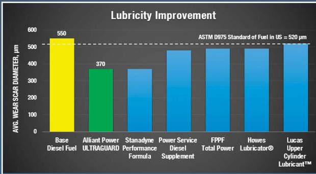
Increasing lubricity will reduce the average wear scar diameter of base fuel resulting in minimized friction and wear of critical fuel system components.
