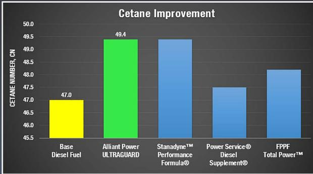
Improving cetane of base fuel will shorten ignition delay periods and will improve engine combustion, faster cold starting, and smooth engine running.
