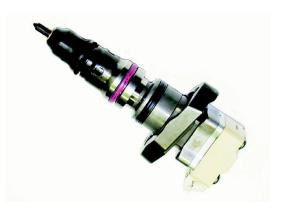
If your customer brings you an injector with a split or cracked nozzle tip, to avoid repeated failures we strongly suggest you treat the failure before you replace the injector. Of the two split or cracked tips warranty claims processed in 2003, both were found to be no fault of the injectors – one failure was tracked to air in the fuel, the other instance was due to low fuel pressure. See Alliant Power Technical Bulletin APTB 03/04 for more detail on preventing injector tip failures.
