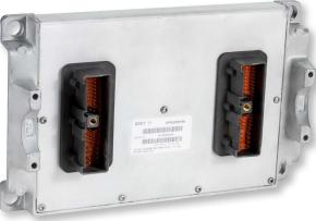
Detroit Diesel ECMs require programming that is specific to the customer's engine and vehicle configuration. The following information must be provided at the time of purchase to receive a pre—programmed ECM.
