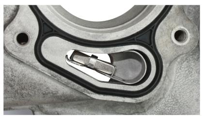
After proper placement of new magnetic filter, install the correct Alliant Power HPOP for the application being repaired. Refer to appropriate engine service manual or equivalent for detailed assembly instructions and torque specifications.
