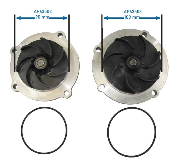
Caution: Both pumps have the same bolt pattern but different sealing areas. As a result, the original pump AP63502 could be inadvertently installed in place of a newer pump AP63503, likely resulting in coolant leakage and engine overheating. Because of different sealing areas, the new pump cannot be installed in place of the original pump.
