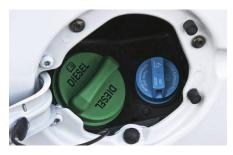
DEF into the fuel system is still a possibility. Caps are color coded blue to
