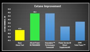
Improving cetane of base fuel will shorten ignition delay periods and will improve engine combustion, faster cold starting, and smooth engine running.
