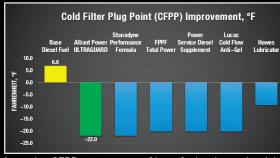
Lowering CFPP temperature of base fuel reduces the risk of fuel gelling and provides superior cold starting and cold weather engine performance.
